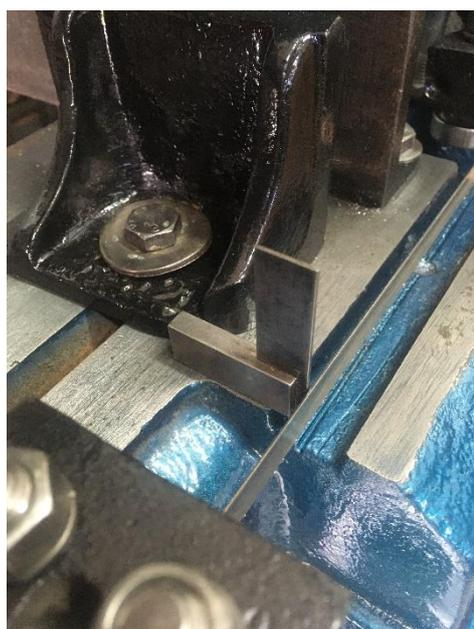
Set the guides as far apart as possible, then slightly rotate each guide block to ensure that the blade is set vertically to the bed of the machine. Do this with the saw body in the horizontal position. It is always wise to set the guides back to close to the job to be cut, or in the vicinity of the vice.
