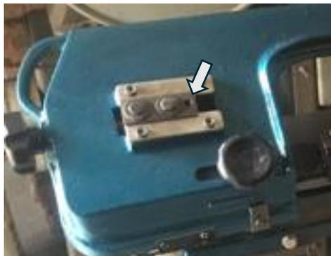
Slacken the blade and re-install the guide blocks.
