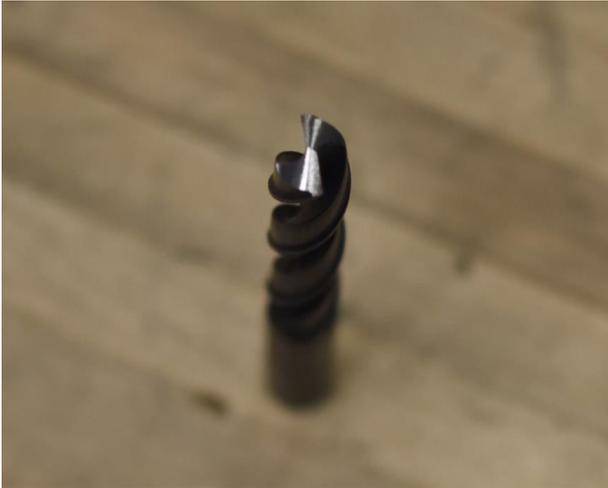
That's normal and requires a lot of patience. But keep on trying! Often rotate which side of the bit you are working on so that you don't favour one side over the other. Always make deliberate cuts, don't try to "feather" a sharp tip by pressing the drill bit lightly into the sander or grinder. This almost always leads to uneven lips or will cause you to roll your lip so that it no longer cuts.
