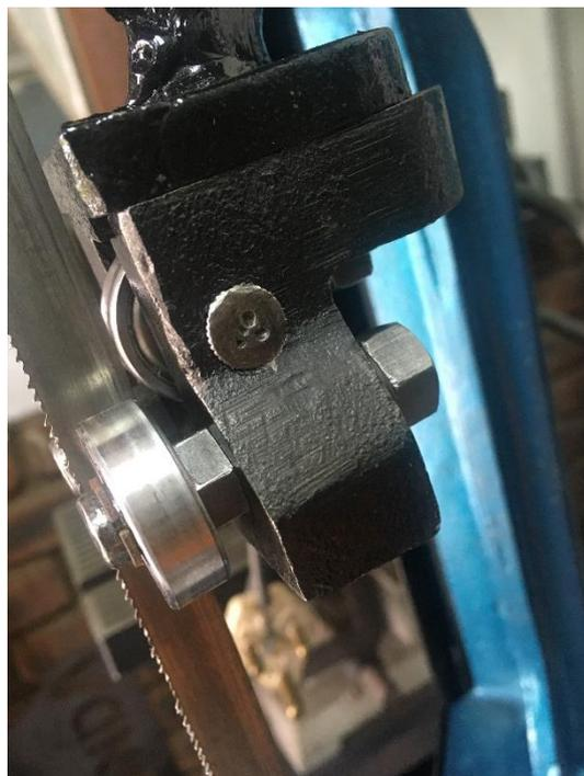
After tensioning the blade until it only just begins to strum, adjust the guide blocks to allow the rear bearing roller to just touch the spine of the blade, do this with both blocks and ensure that there is no pressure from either.
